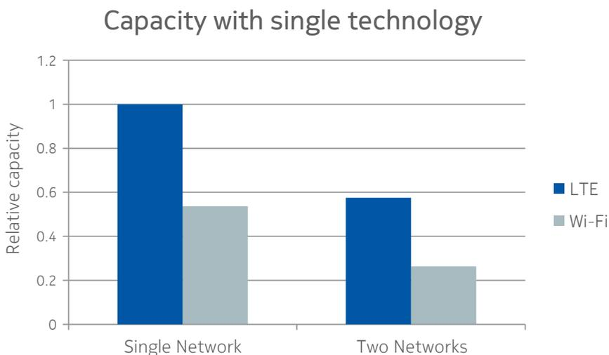
Figure 7. Performance per access node with two LTE or two Wi-Fi networks on the same channel
