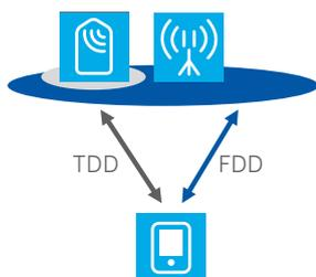
Figure 4. LTE-Advanced aggregation between FDD and TDD bands.
