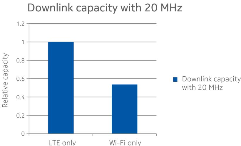
Figure 6. LTE capacity compared to the Wi-Fi capacity in the office environment.
